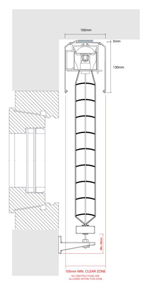
Elevation and Plan - Dimension and Clearance Allowance Ref: VA3010a
