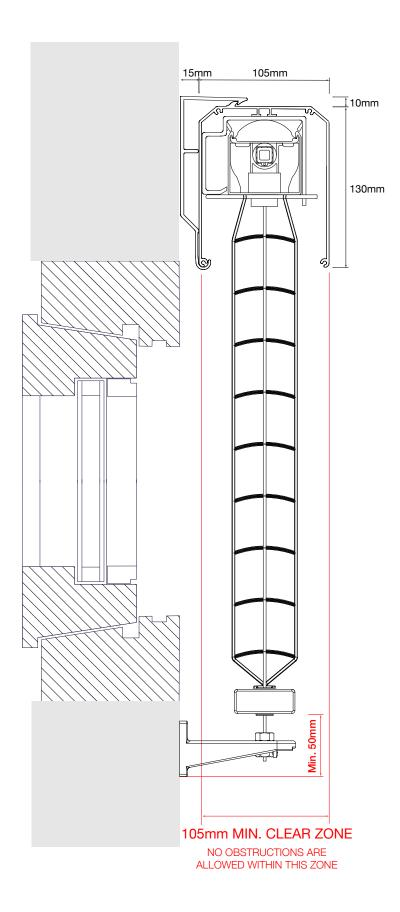
Recess Fitted Example with Wire Guides *Ref: VA3002a*
