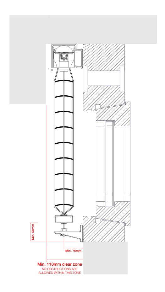
Top Fitted Example with Cassette D Pelmet and Wire Guides Ref: VA3003a
