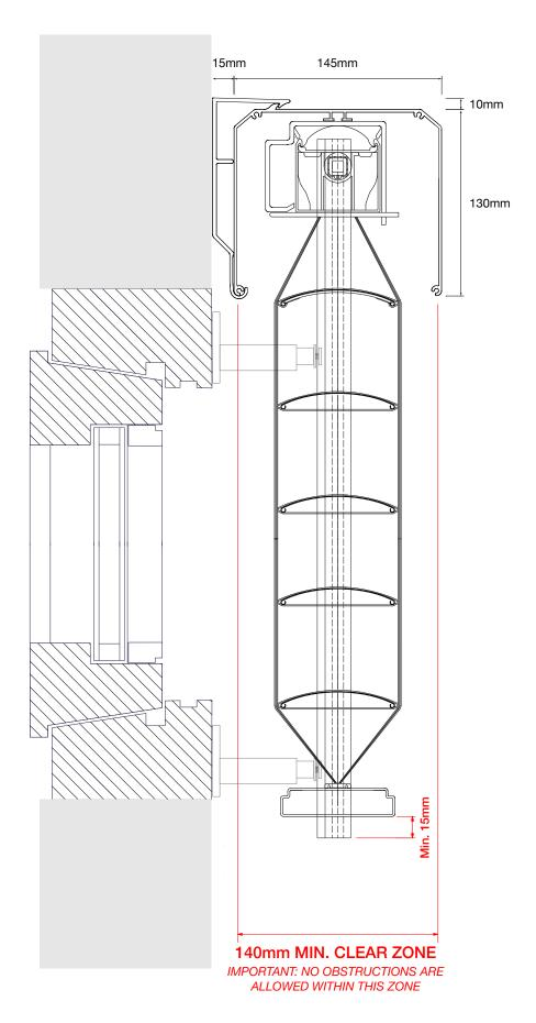
Recess Fitted Example with Extruded Guides Ref: VA0002b
