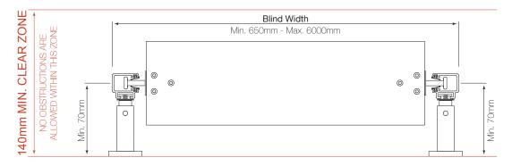
Elevation and Plan Dimension with Clearance Limits *Ref: VA0010c*
