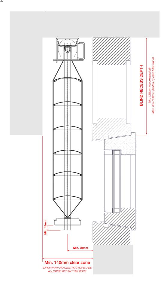
Top Fitted Example with Cassette B Pelmet and Extruded Guides *Ref: VA0003b*
