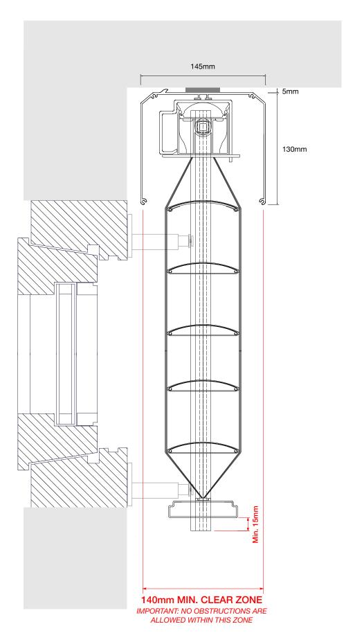
Plan Dimensions and Clearance with Extruded Guide Rails Ref: VA0009b
