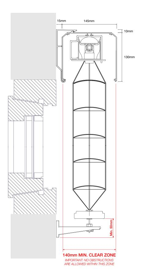
Recess Fitted Example with Wire Guides Ref: VA2002a
