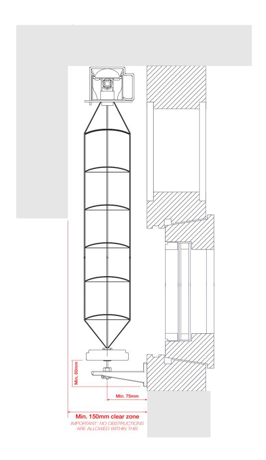
Top Fitted Example with Cassette B Pelmet and Wire Guides Ref: VA2003a
